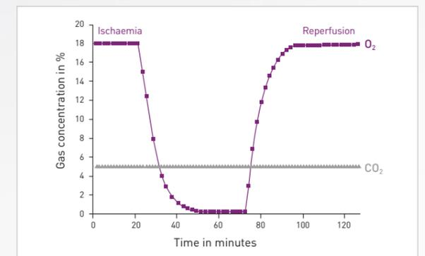
Example of O<sub>2</sub> deprivation and reoxygenation (down to 0.2% O<sub>2</sub>; purple) with steady 5% CO<sub>2</sub> (grey) performed by the CLARIOstar with ACU.
